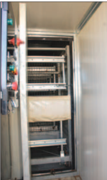
KEEPING TABS: A user door allows the grower to take a look into the barn as the cure progresses.
