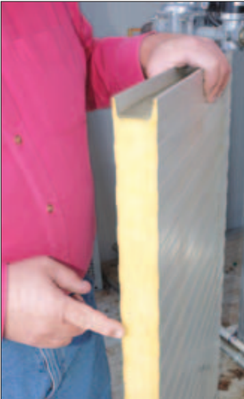
COZY COAT: Two inches of insulation keep warmth inside the barn.
